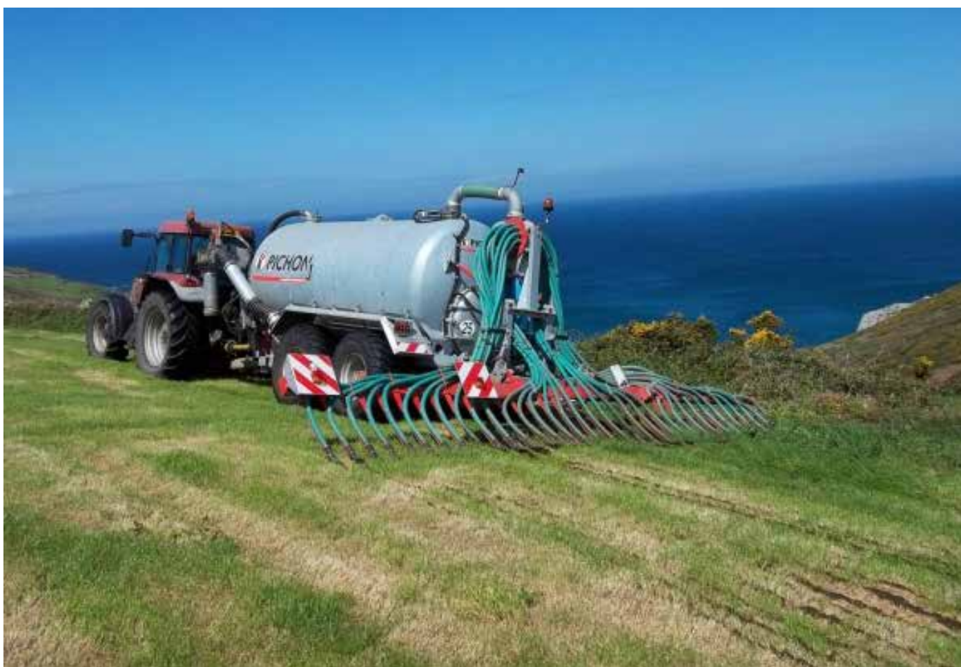
Figure 1: Apply slurry via a low trajectory spreading technique to reduce nitrogen loss and improve efficiency
