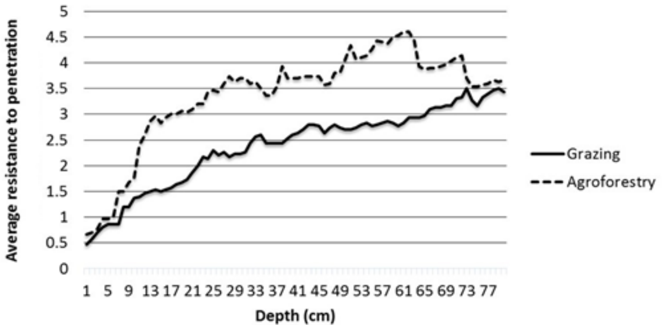
Fig 1. Infiltration potential is greater in the agroforestry, creating a soil profile more resistant than a grassland system.
