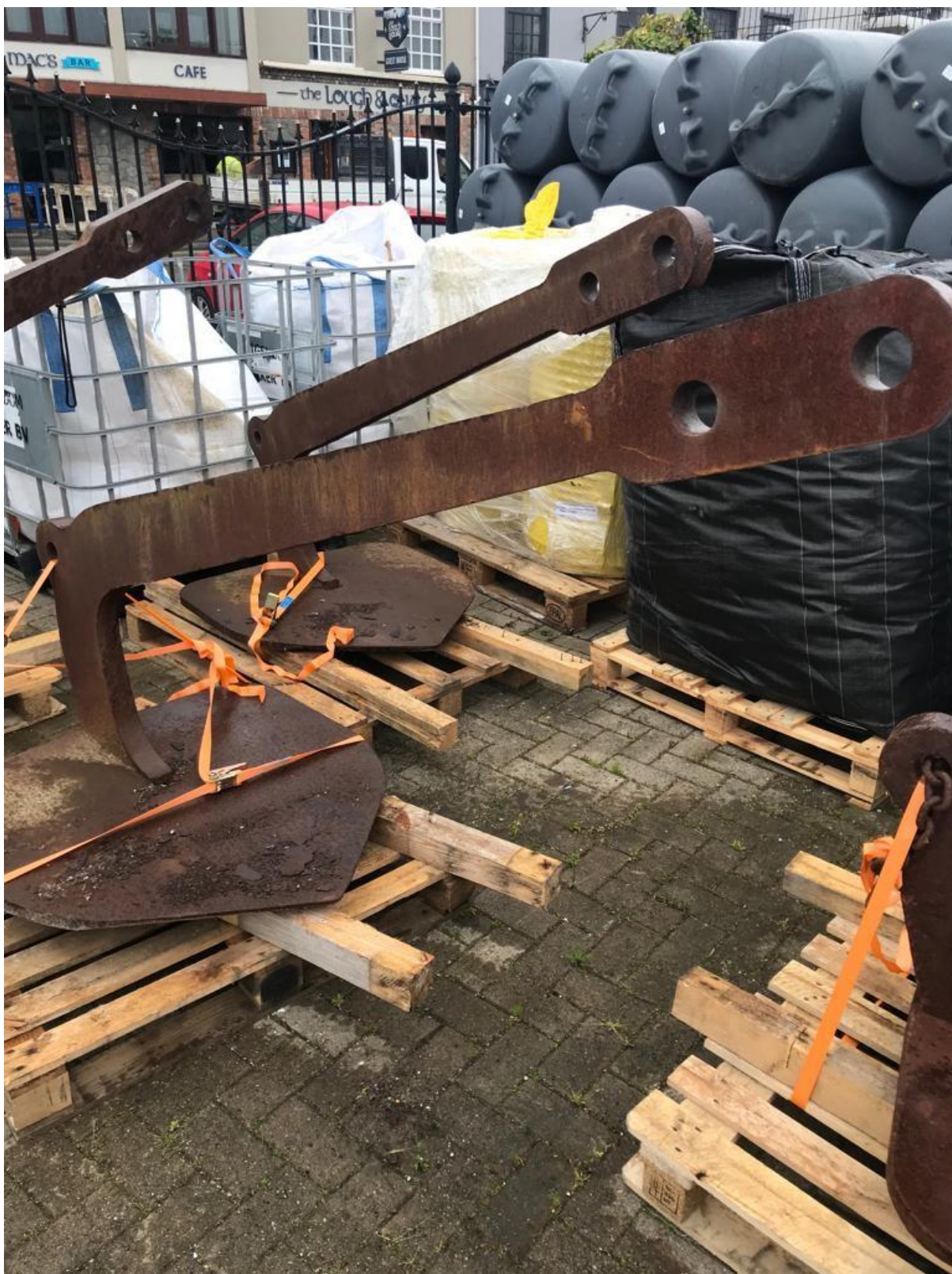
Figure 7: Photo showing the anchors to be deployed as part of the trial spat collector system.
